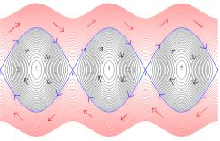
Orbit of damped pendulum.
