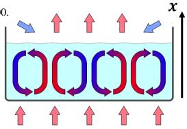
As  $\Delta T$  is further increased the complexity and the number of convection rolls increase until a critical moment is reached and chaos sets in. This irregular and chaotic motion is studied by looking at the Fourier-transform of the fluid motion in the *x*-direction. This way multiply periodic beavior can be distinguisged from chaos
